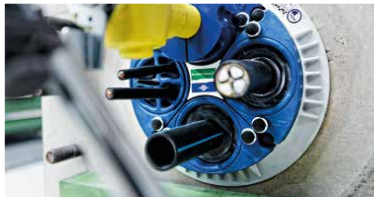
Load limits test on multi-utility building penetration
