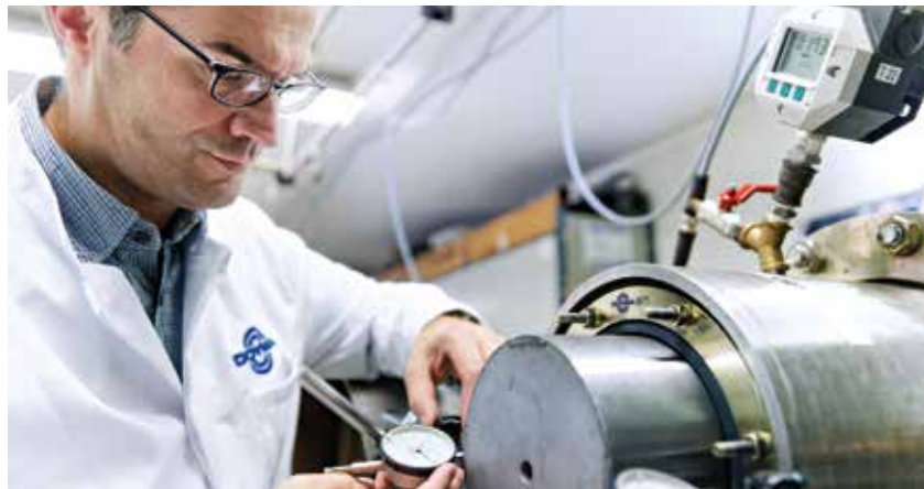
Slip limit test on a sealing gasket
