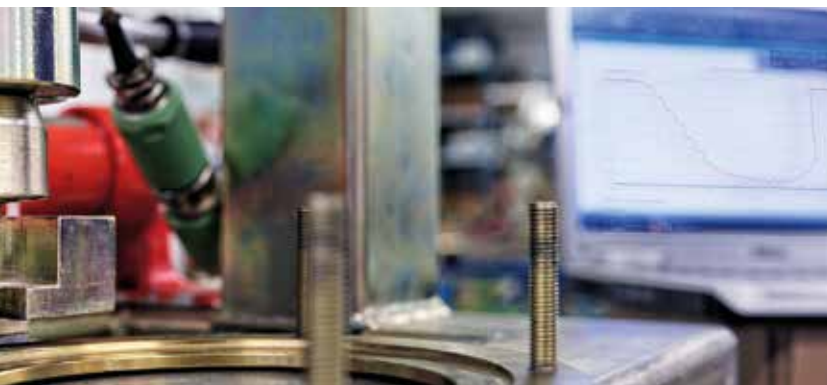
Pull test of a bolt with a gradient
